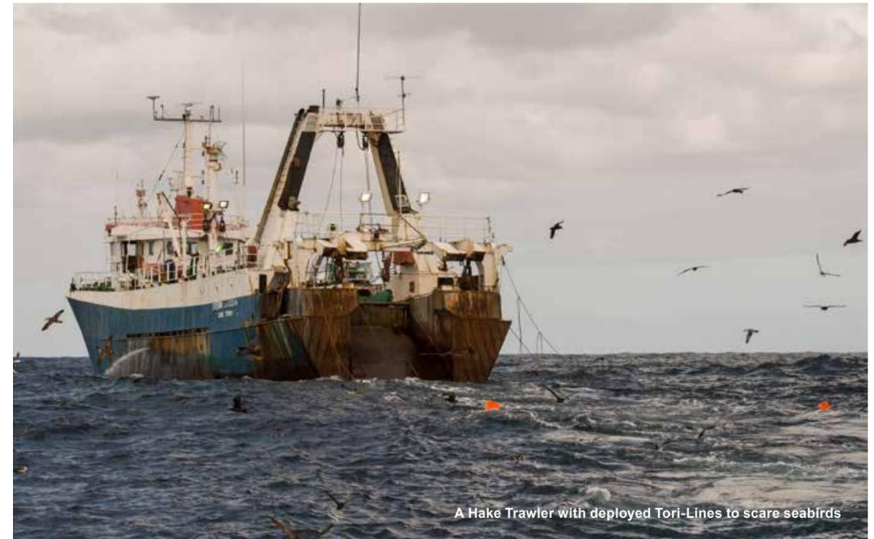
A Hake Trawler with deployed Tori-Lines to scare seabirds
